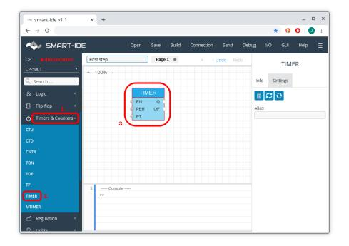
Block "Timer" can produce periodic pulses with desired period. We will use it to periodically click with the relay output. Now click on category "In / out" and drag block "INPUT" to the drawing surface. In the right panel, there are options of the selected block. Click on "Constant" and set value to 1000. We want our timer to work with period of 1000ms.
