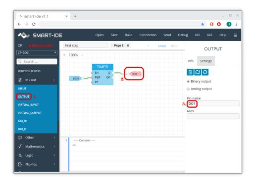
Now we have a timer that generates periodic 1s pulses, that feed relay output. It's a time to test our project. Click on the "Build" item in the top menu, the project should be compiled. If you are not connected to the PLC, click on the "Connect" button in the right panel. Now click on the "Send" item and the project should be sent to the PLC.
