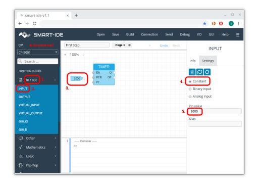
Now drag the bullet of our block "1000" to the bullet of timer's "PER" input to connect them with a net. From the left panel, drag block "OUTPUT" to the drawing surface. In the right panel, set pin name to "DO1". This should be the first relay output of our PLC. Drag the bullet of our block "DO1" to the bullet of timer's "Q" output.
